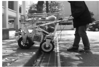
Fig. 4(c). Rear wheels climbing up the curb.
