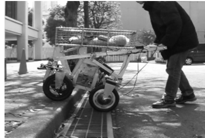
Fig. 4(b). The carriage being driven until the rear wheels meet the curb.
