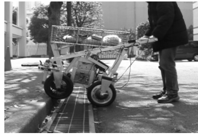
Fig. 4(a). The front wheels climbing up the curb.
